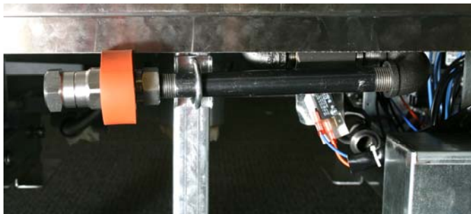
Figure 7: The plumbing with the brace and the quick disconnect installed is shown above.
