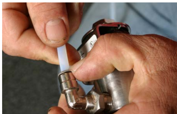
Figure 3: Release the solenoid vent tube by depressing the collar on the coupling.
