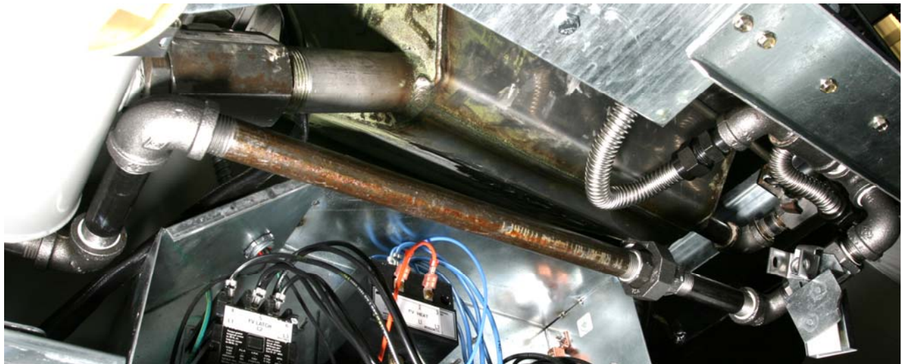
Figure 9: The completed plumbing for front disposal is shown. Install the rear section, including the half union, first. Install the front bracket and the rearward junction, leaving the junction loose.
