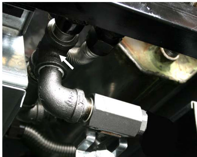
Figure 2: This tee (see arrow) may be present and plugged in newer fryers.
